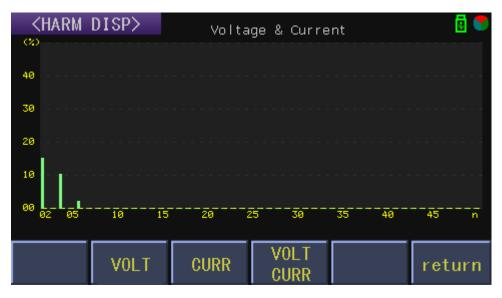
Figure 4-10 Bar graph display for Harmonic display interface
