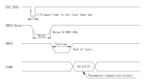
Figure 10-1 Handle timing diagram
