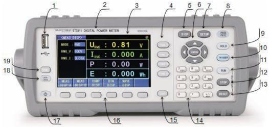
Figure 2-1 shows the front panel of ST33XX.
