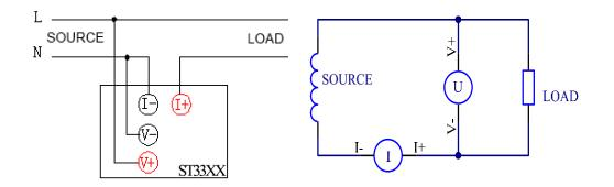
Figure 6-2 External connecting method ----- suitable for large current
