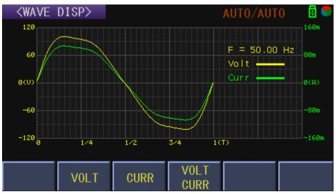
Figure 4-12 Input waveform with harmonic components
