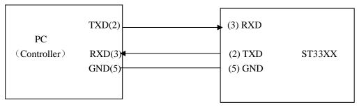
Figure 8-1 Connection of the instrument with PC
